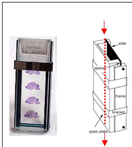
**Figure 4:** GenePaint Flow Chamber with slide carrying tissue sections (purple) after *in situ* hybridization. Schematic drawing shows how the slide is assembled in the flow chamber.
