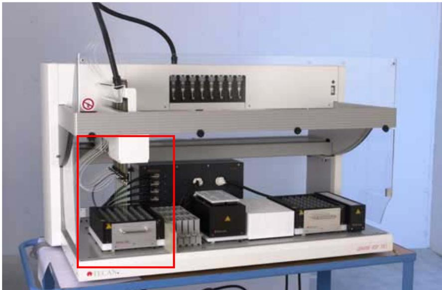
**Figure 1:** GenePaint System on a GENESIS RSP 150/8 Platform. Visible from left to right are: GenePaint Chamber Rack, 15 small reagent reservoirs, four medium-size heatable reagent reservoirs, three large reagent reservoirs, another GenePaint Chamber Rack, and a heatable rack for Eppendorf tubes.
