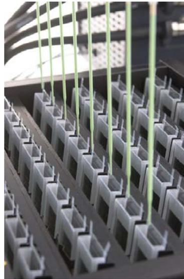
**Figure 3:** Close-up of GenePaint Flow Chambers located in the GenePaint Chamber Rack. At their backs the flow chambers are in direct contact with the heat exchange wall. The eight pipet tips above one row of flow chambers are visible in green.
