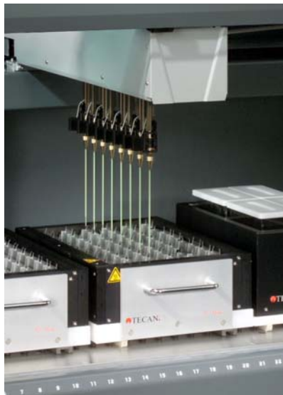
Figure 1: GenePaint Chamber Rack holding 48 Flow-Through chambers. The Liquid Handling arm of the robotic system is equipped with eight dispensing tips. It assures automatic and parallel pipetting of all solutions.
