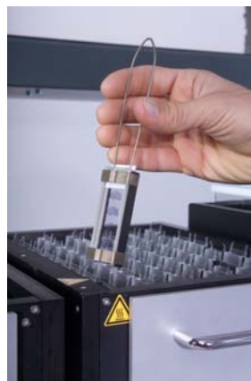
Figure 2: GenePaint Flow Chamber with slide carrying tissue sections. Schematic drawing shows how the slide is assembled in the flow chamber.
