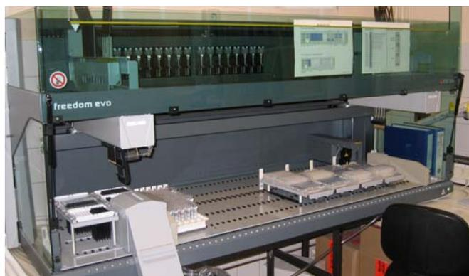
**Fig. 1. Freedom EVO configuration.** Two liquid handling arms for alternative use of fixed or disposable tips. The arm for DiTis is equipped with the lower DiTi eject option to minimize the risk of cross-contamination.
