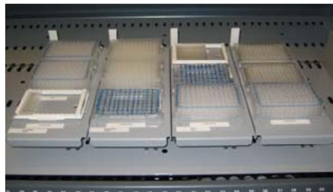
**Fig. 4. Sample distribution.** The destination area has space for 12 microtiter or deep-well plates, allowing the pipetting of all of the required range of diagnostics assays as well as preparing the sample archive plates.
