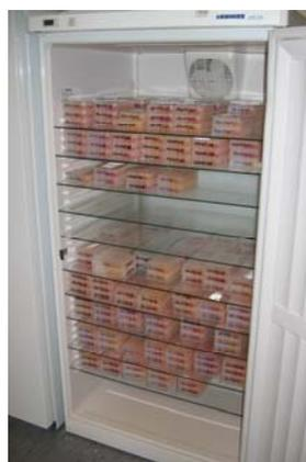
**Fig. 5. Sample archiving.** Deep-well plates can be stacked for archiving, significantly reducing the required storage space.
