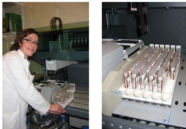
**Fig. 3. Loading area.** Liquid level and clot detection ensures safe sample transfer.
