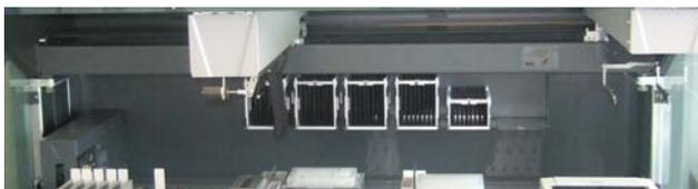
**Fig 4** Additional storage places for consumables save space on the worktable. The flexible number and size of shelves allow initial loading of necessary consumables such as DiTi box carriers, microplates and deep-well plates to reduce operator actions during processing.
