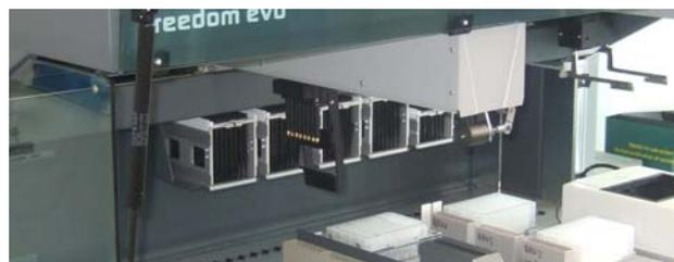
**Fig 3** Safety: the lower DiTi eject option enables smooth dropping of used disposable tips directly into the waste. The risk of splashing remaining liquid droplets while dropping the tips from the tip adapters is avoided.
