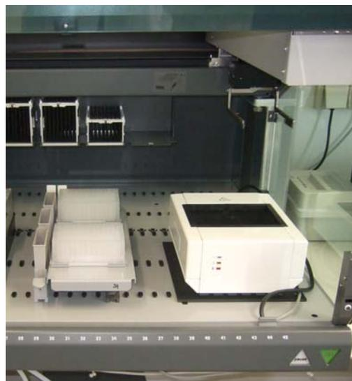
**Fig 5** Complete process automation. The diluted serum is pipetted into the deep-well plate and lysis buffer is added. The lysis can be carried out on the worktable at room temperature or in a heated incubator. Here a third party microplate incubator from Biostep, GmbH (Jahnsdorf, Germany) was integrated to reduce manual sample handling and to increase the workflow efficiency.
