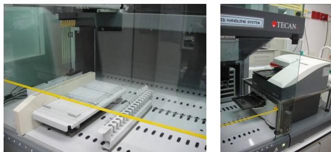
Figure 3 Detailed view of the loading area (left); reader and washer are integrated on the right hand side of the platform (right)
