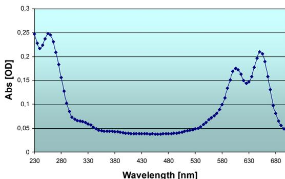
**Figure 4:** Absorbance scan of Cy5 labeled cDNA probe. Scan from 230 – 700 nm, bandwidth 5 nm, raw values are plotted (non referenced, non-blanked) for generating the curve. Note that Cy5 has two absorbance peaks (605 and 649 nm).
