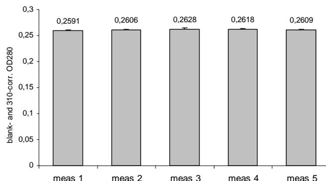
**Figure 2:** Measurement reproducibility of 5 individual samples on the NanoQuant Plate
