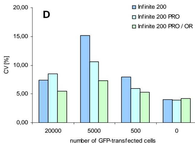
Figure 2: Well-to-well Uniformity. (A) 4 flashes per well, (B) 12 flashes per well, (C) 25 flashes per well (default), (D) 40 flashes per well. The measurements were performed on an Infinite 200 with a standard FI bottom option, an Infinite 200 PRO with the enhanced FI bottom modul and the Infinite 200 PRO / OR were done with enhanced FI bottom with the Optimal Read (OR) function. Values represent average signals of 24 replicate wells.
