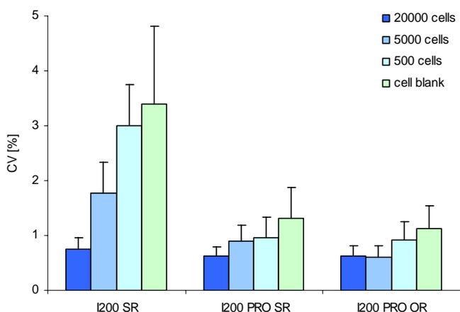
Figure 3: Measurement reproducibility. The measurements were performed on an Infinite 200 with Single Read (SR) and on an Infinite 200 PRO with Single or Optimal Read (OR). Values represent average signals of 24 replicate wells that were measured 5 consecutive times plus StDev. The CV values refer to the variation between all five measurements.
