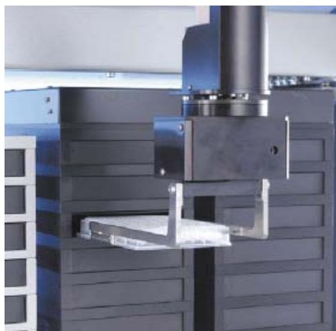
**Figure 4-4:** RoMa arm loading a robotic-compatible 37°C incubator
